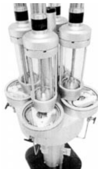
Fig. 2 Powder feed system for four powders by Medicoat AG
